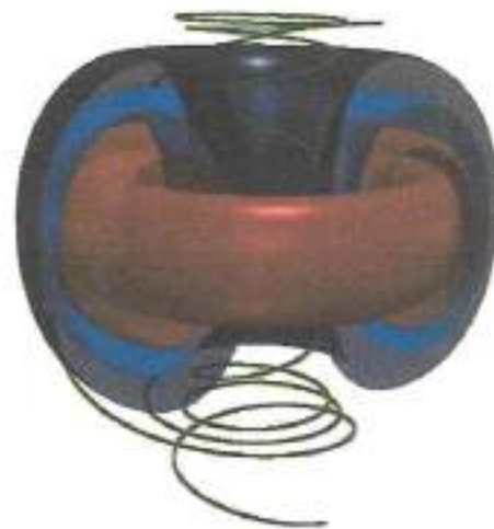
Figure 1: Pressure isosurfaces and magnetic field line for MHD equilibrium in a ST configuration with A \sim 1.6 , I_p = 1.3\text{MA} and \beta_n \sim 0.35 .
